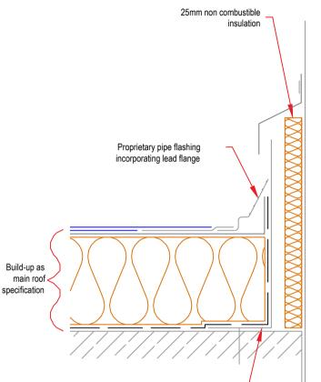
0.9mm galvanised metal pipe sleeve mechanically fastened to the roof deck
